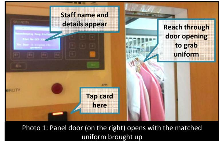
Photo 1: Panel door (on the right) opens with the matched uniform brought up
